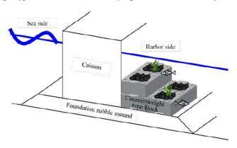
Keywords: tsunami, extremely big waves, breakwater reinforcement, counter-weight type block, friction factor, tsunami overflow
