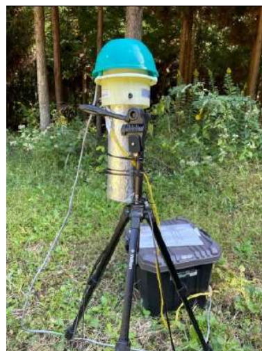
Photo 4 Test observation of air temperature and humidity sensor with forced ventilation system.
