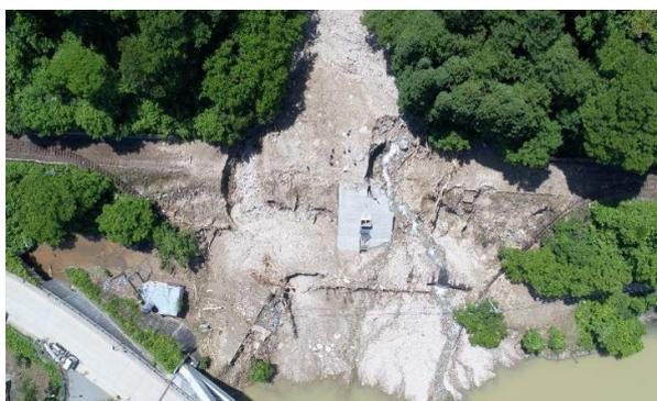
Fig. 1 Sediment disaster of the JR Takayama Mainline in Hida City, Gifu Prefecture<sup>6)</sup>
