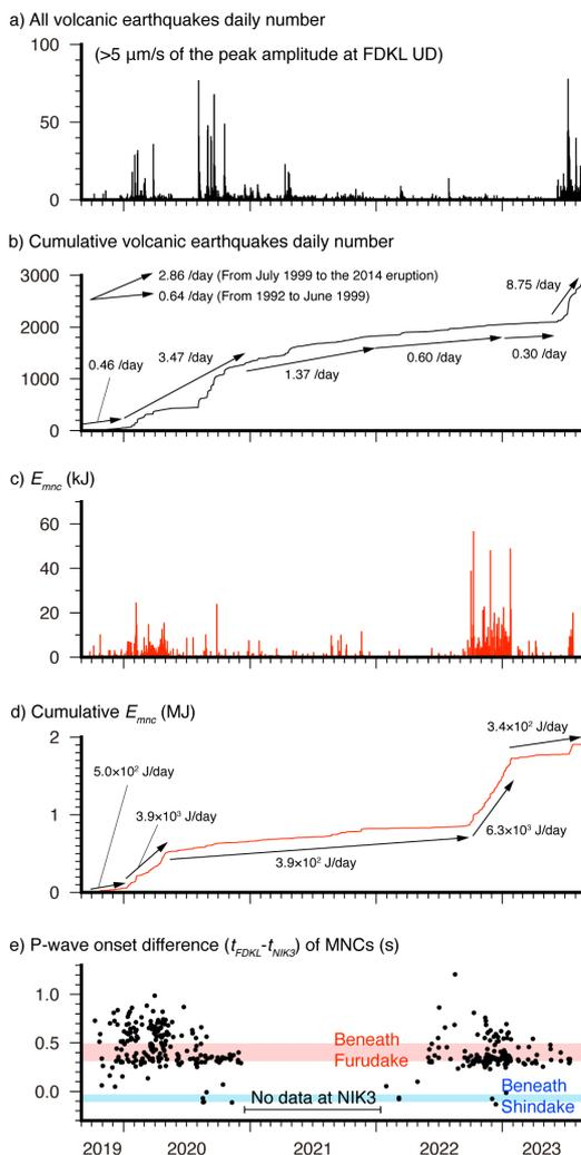
Fig. 6 Time series of (a) daily number of all volcanic earthquakes, (b) seismic energy of each MNCs ( $E_{mnc}$ ), (c) cumulative daily volcanic earthquake number and  $E_{mnc}$ , and (d) P-wave onset difference between FDKL and NIK3 ( $t_{FDKL} - t_{NIK3}$ ) from September 2019.
