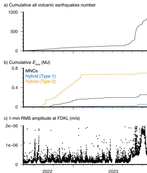
Fig. 11 Time series of (a) cumulative daily number of all volcanic earthquakes, (b) cumulative  $E_{mnc}$ , and (c) 1-min RMS amplitude at FDKL in the period September 2022 to August 2023.
