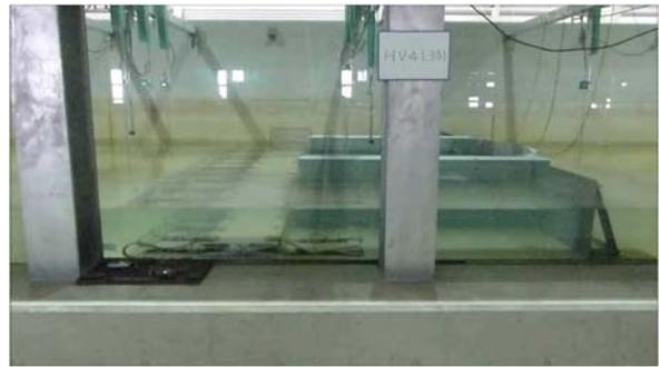
Photo 15 Experiment for effect of Fin-type movable breakwater to reduce tsunami force acting on visor gate
