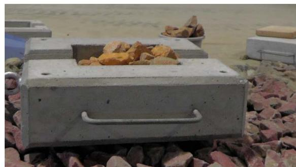
Photo 10 Towing test of Counter weight block
