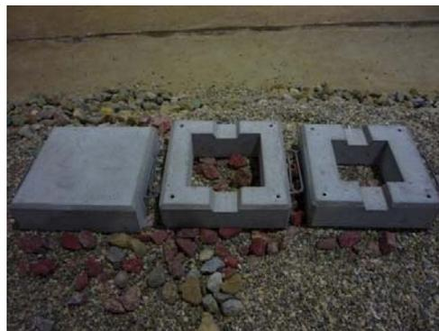
Photo 9 Comparison of Plane and Counter-weight blocks
