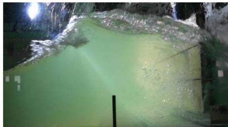
Photo 16 Stand-up of Water defense door on tsunami attack
