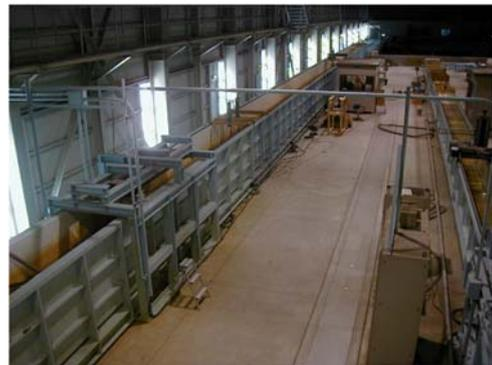
Photo 7 45m Multi-purpose directional random wave generation channel (UOL) (by UOL homepage)
