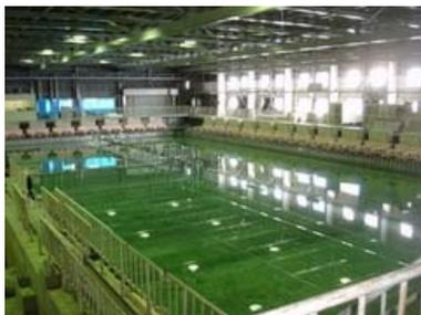
Photo 4 Dual-Face Serpentine-type Wave Maker
