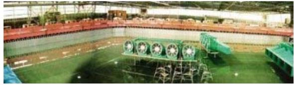
Photo 5 Intelligent Directional Wave and Current Generator
