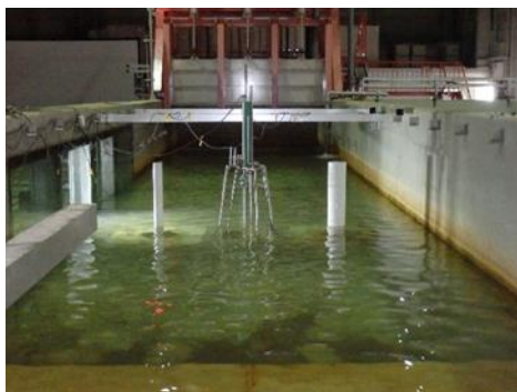
Photo 2 View of Model Mono-Pile (Left side; \phi=6\text{m} , Right side, \phi=12\text{m} )
