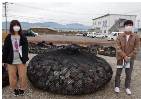
Photo 1 Overview of Flexible Anti-Scouring Unit
