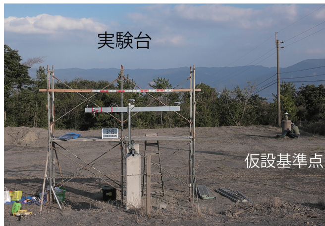
Fig. 7 The platform at work. The platform is on the left. The current reference station KURB on the right
