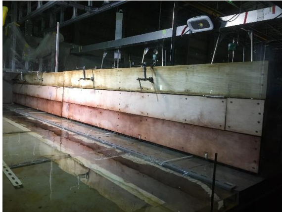
(2) "Anti-tsunami Door" on tsunami attack
