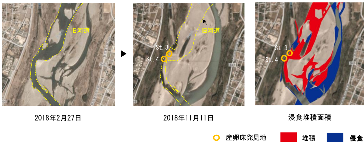
Fig. 30 Erosion deposition area (Right bank sand bar at from 17.4 km to 14.2km)
