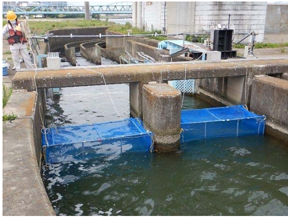
Fig. 8 Situation of capture by customized net for Fishway
