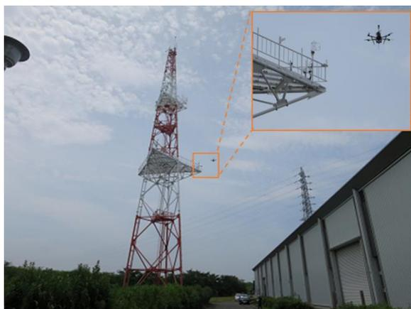
Fig. 11 Hovering drone at Site B nearby meteorological observation tower equipped with ultra-sonic anemometer.
