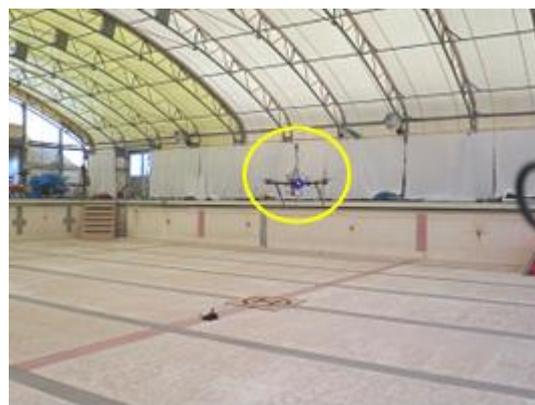
Fig. 3 Hovering drone installed with ultra-sonic anemometer at 2 m from floor.
