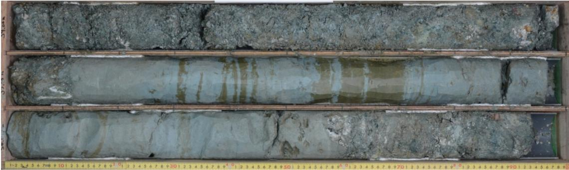
Photo 2 Example of boring core (depth 54m-57m).
