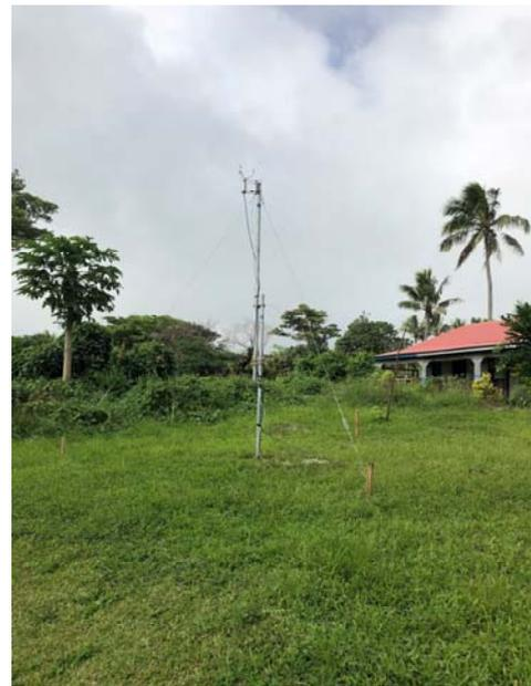
Photo 1 Ultrasonic anemometer installed in Vanuatu
