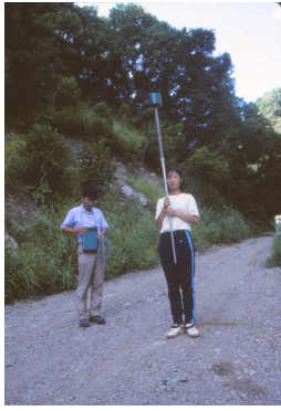
Photo 1. Profile survey of the geomagnetic total intensity across the Atotsugawa fault.
