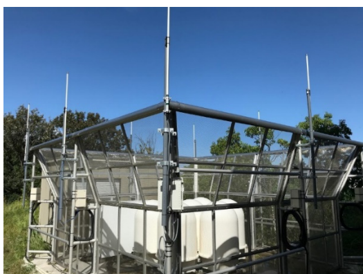
Photo 1 Wind Profiiler (Above) ,Sub-array antennas.
