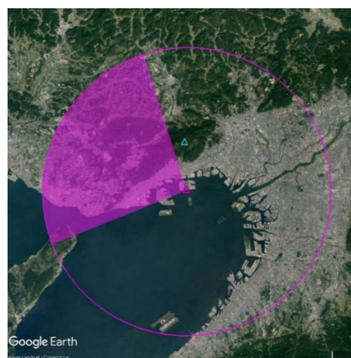
Fig.4 Ka-band radar Observation area in Sector-PPI scan.
