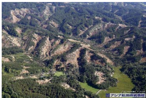
Fig. 1 Landslides of pyroclastic fall deposits in Atsuma induced by the 2018 Eastern Iburi earthquake. Photo by Asia Air Survey Co., Ltd. and Aero Asahi Corporation.
