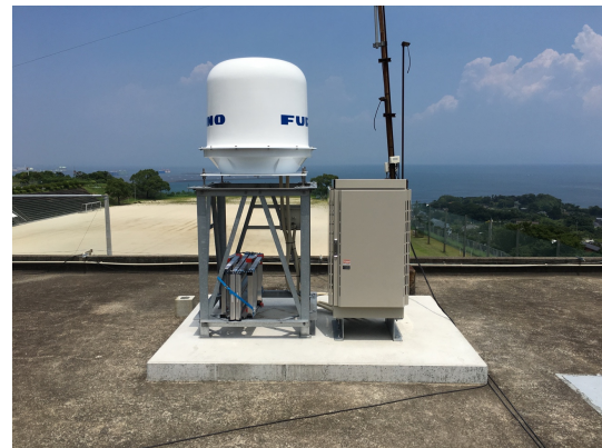
Photo 1 Small-size X-band multi-parameter wether radar at Kinkowan High School
