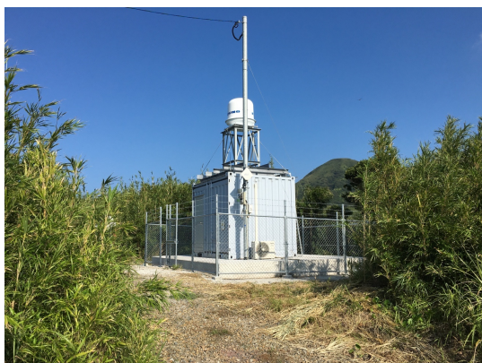
Photo 2 Small-size X-band multi-parameter wether radar at Suwanosejima volcano
