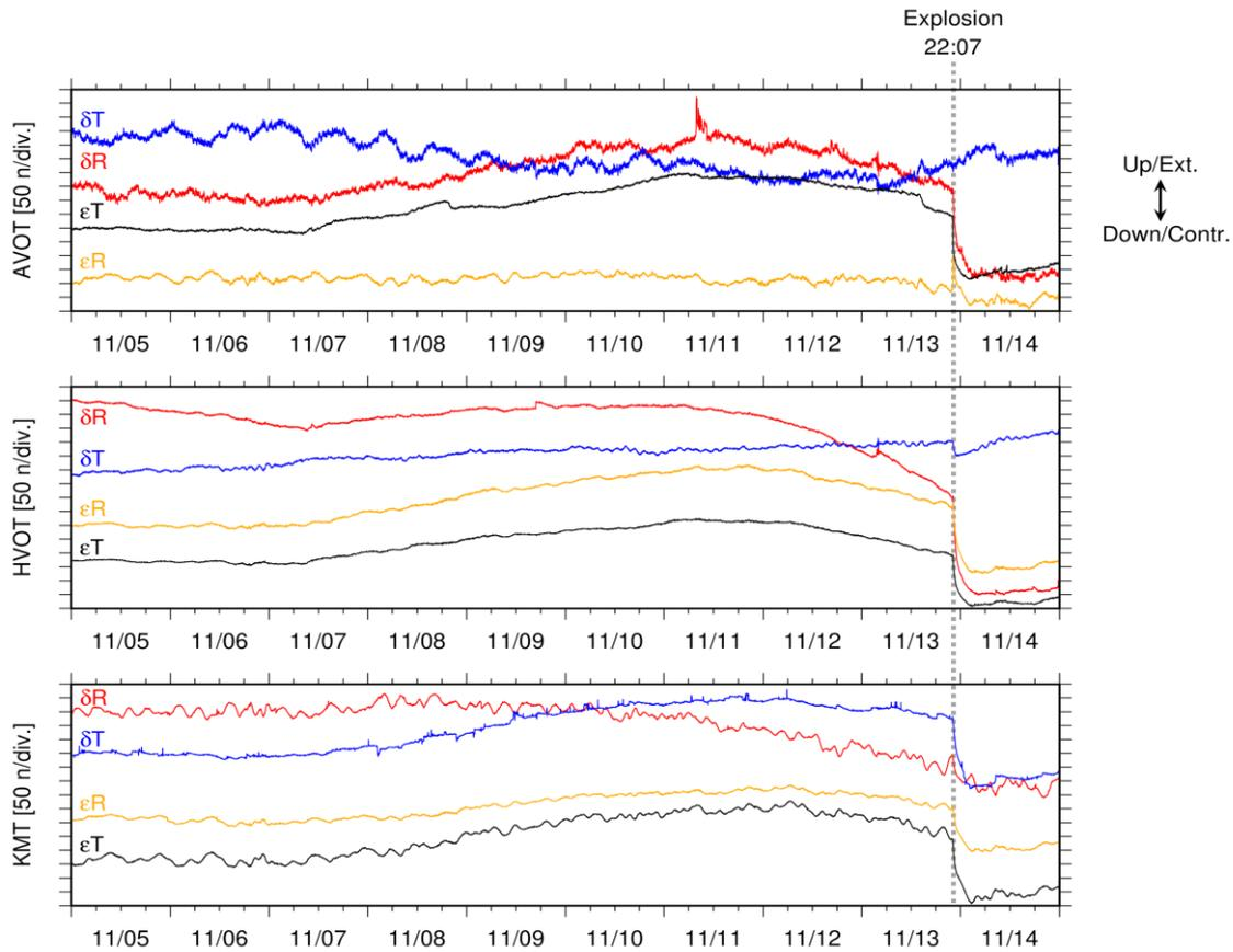
Fig. 2 Tilt ( $\delta$ ) and strain ( $\epsilon$ ) records at each observation tunnel during the period of November 5–14, 2017. The radial (R) component is positive toward the summit crater of Minami-dake, and the tangential (T) component is positive in the direction rotated clockwise by  $90^\circ$  from the radial component, respectively. The gray dashed line represents the onset of explosion at Minami-dake on November 13, 2017.
