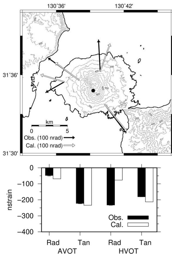
Fig. 4 (top) Location of obtained Mogi source (the solid circle) and comparison of observed (black) and calculated (white) tilts. Error ellipses are  $1\sigma$ . (bottom) Comparison of observed (black) and calculated (white) strain changes. Error bars are  $1\sigma$ .
