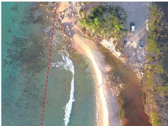
Photo 2: Coastal erosion at Frederiksted in St. Croix (red line corresponds original shoreline)
