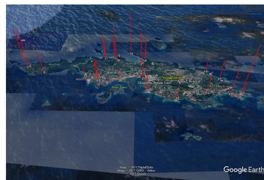
Fig.3: Measured inundation and run-up heights around St. Thomas (maximum height is 6.4 mF)
