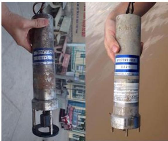
Fig. 9 Salinity (left) and turbidity (right) meters
