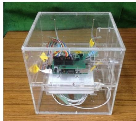
Fig. 6 Prism for pressure sensors' test
