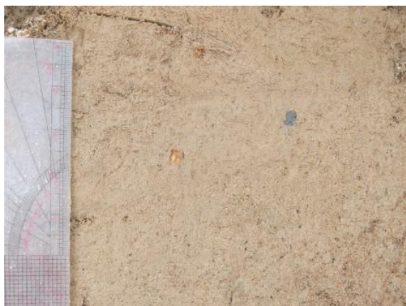
Fig. 19 Hydrothermally altered pink gray volcanic ash, which contains pumice grains (SWT-1).
