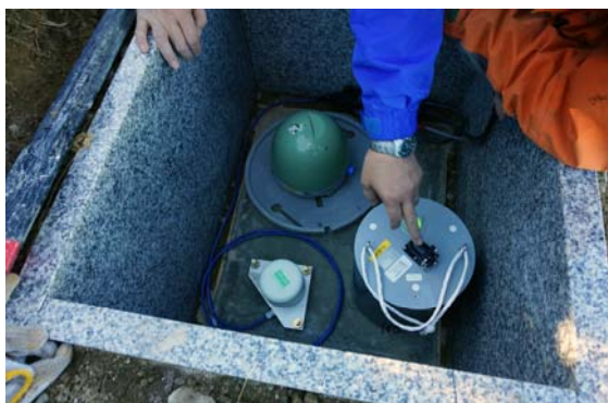
Photo 1: (a) (upper) Newly constructed DP.NKOT (Nakao-Toge pass) station. Main part of the equipment (left), GNSS antenna pillar, (middle right), and a pillar for the proton precession magnetometer (right) are seen. (b) (lower) Instruments installed at DP.NKOT. Broadband (upper left) and short period (right) seismometers, and tiltmeter (lower left) are seen.
