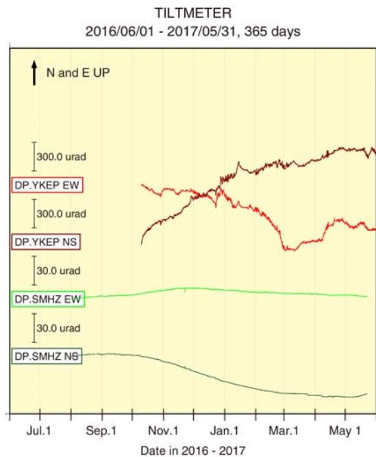
Fig.4 : Tilt record at stations DP.YKEP and DP.SMHZ. Surface type tiltmeter is installed in DP.YKEP site while borehole type instrument are installed in DP.SMHZ site.
