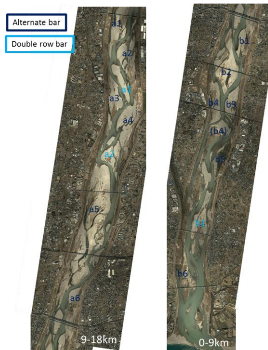
Fig. 21 Alternate bars and double row bars in Tenryu River 0-18km
