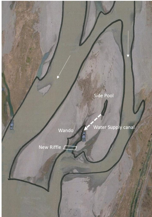
Fig. 8 Location of water supply canal and new riffle
