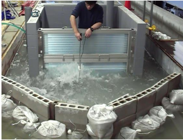
Photo 5 Apparatus for Test (flow).
