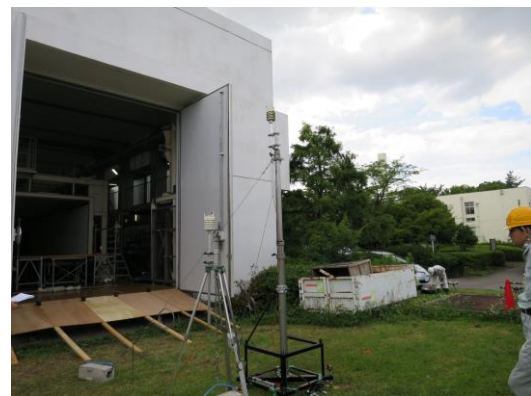
Photo 3 Wind speed distribution observation by supersonic anemometer
