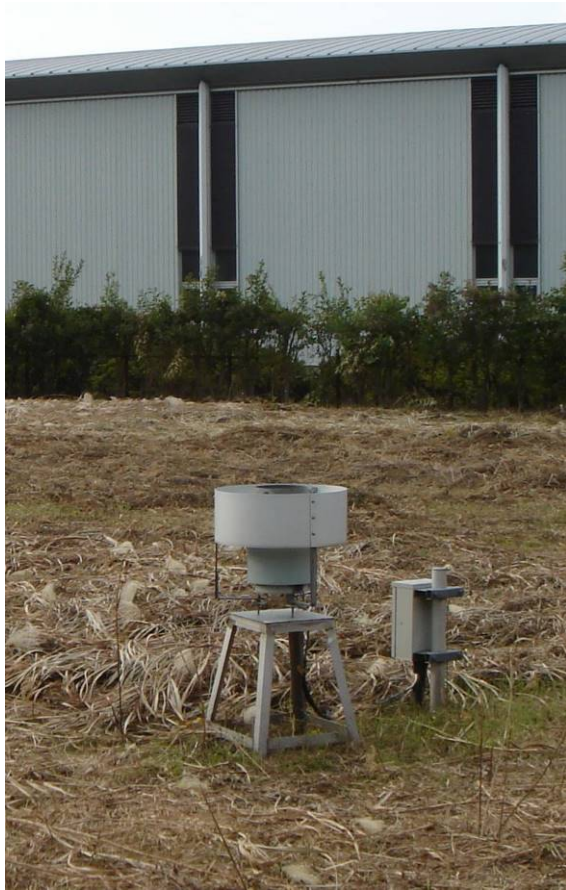
Photo 4 Tipping bucket rain gauge in the field
