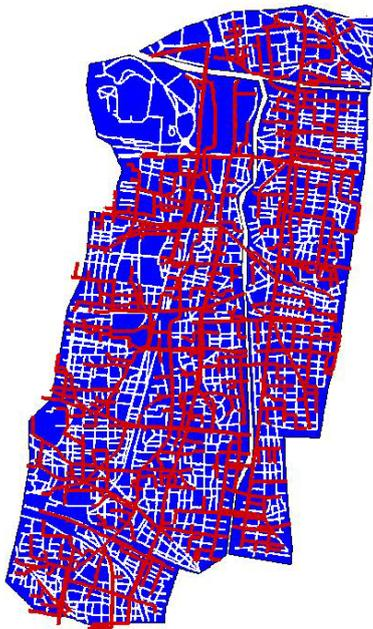
Fig. 4 Arrangement of sewer pipes and storm drains
