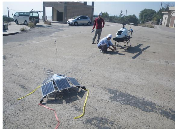
Photo 1 An unmanned autonomous helicopter and a seismic instrument with a solar power unit.
