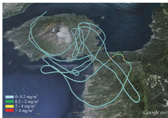
Fig.4 Flight path and ash concentration measured by DustMate on July 27, 2013.
