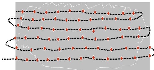
Fig. 1 Conceptual drawing of zig-zag measurement in a cross-section of plume. Red-color diamonds denote measurement points and dash line denotes flight path.
