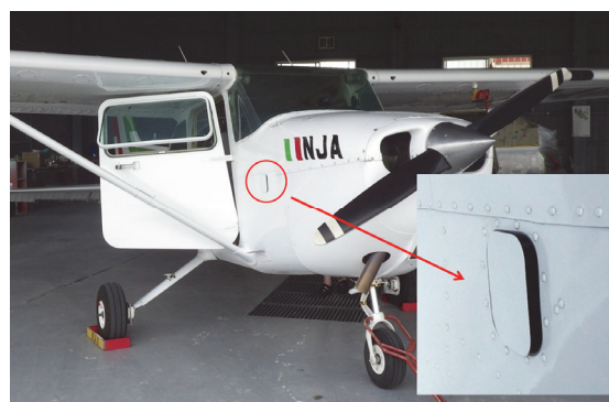
Photo 2 Cessna plane used for airborne measurement and magnified photo of air scoop. This Cessna has the capacity of 4 people and can go up to approximately 2400m attitude.
