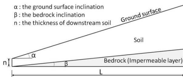
Fig. 3 The simplified bedrock position model
