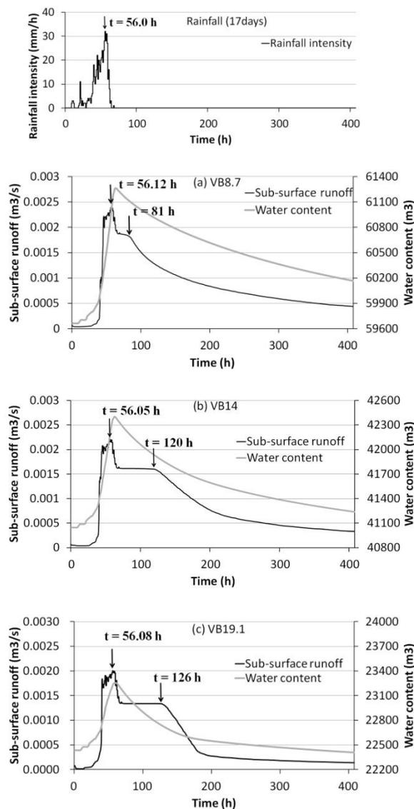
Fig. 6 The rainfall-runoff hydrograph in volcanic debris slope (a)bedrock inclination of  $8.7^\circ$  (b)bedrock inclination of  $14^\circ$  (c) bedrock inclination of  $19.1^\circ$
