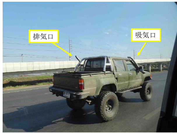
Fig. 16 Automobile with raised air intake and exhaust pipes
