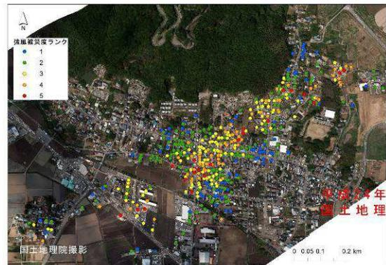
Fig. 6 Distribution of damage in Hojo and Koizumi area
