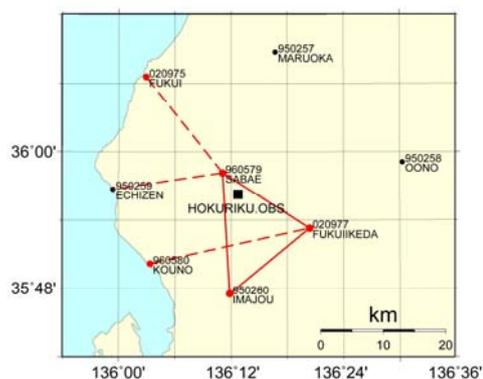
Fig.9 3 big red points : permanent GPS monuments that we used in this study. Black square : Hokuriku observatory in which tunnel the extensometers are set.
