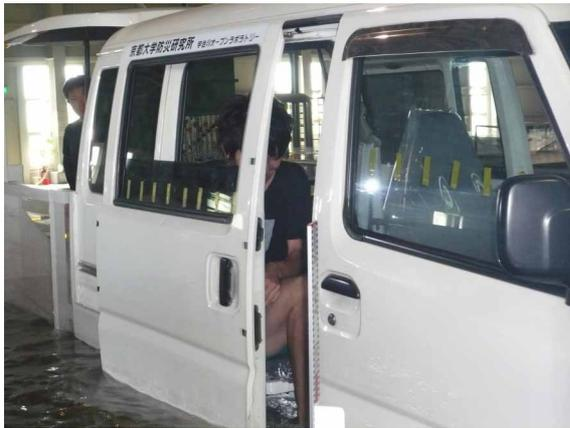
Photo 2 Evacuation experiment (sliding door)
