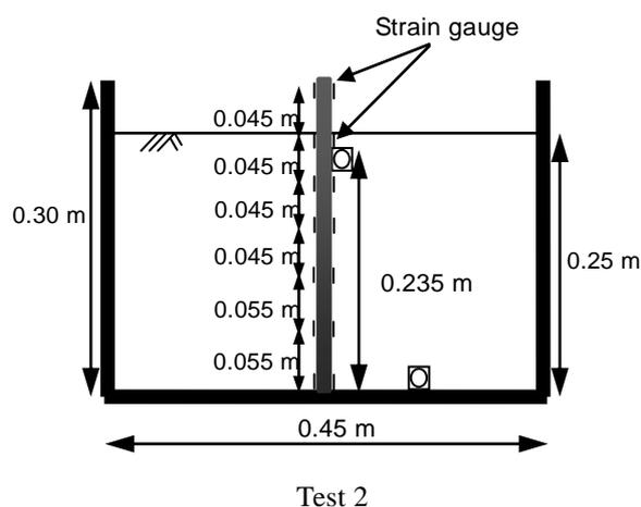
Fig. 5 Illustration of single pile test setup (test 2)
