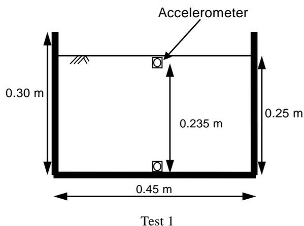
Fig. 4 Illustration of free-field test setup (test 1)
