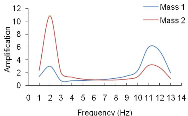
Fig. 11 Fixed base structure amplification versus frequency (test 4): Double degree of freedom
