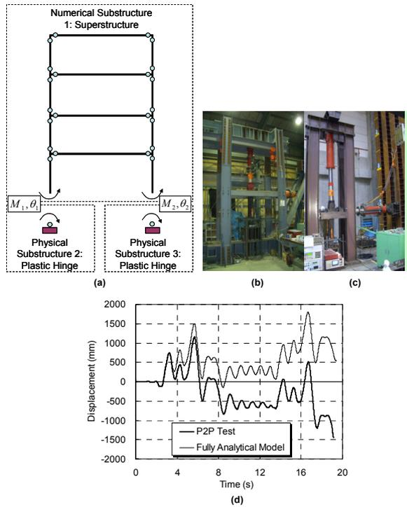
Fig. 10 Four-story steel moment frame: (a) Prototype; (b) and (c) Physical setups in two laboratories; (d) Displacement time histories obtained from test and associated numerical analysis
