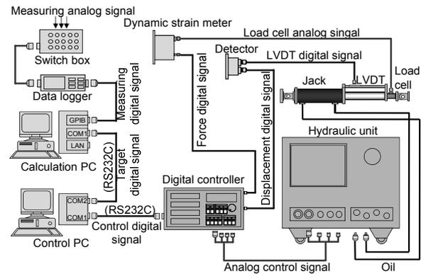
Fig.1 Typical online hybrid test system using conventional loading facilities (External loop)
