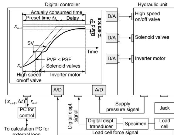
Fig. 3 Feedback control using digital controller (Internal loop)
