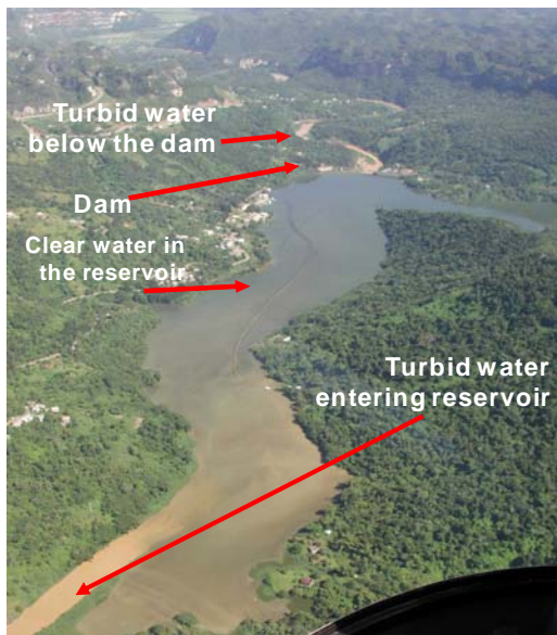
Photo 4 Turbidity current passing through (Morris and Fan, 1998)
