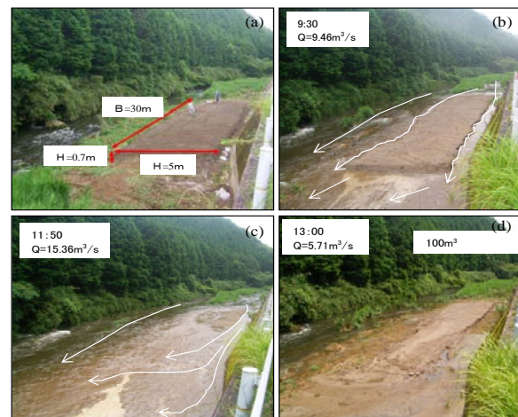
Fig. 16 Processes of erosion and deposition of the placed sediment during flood
