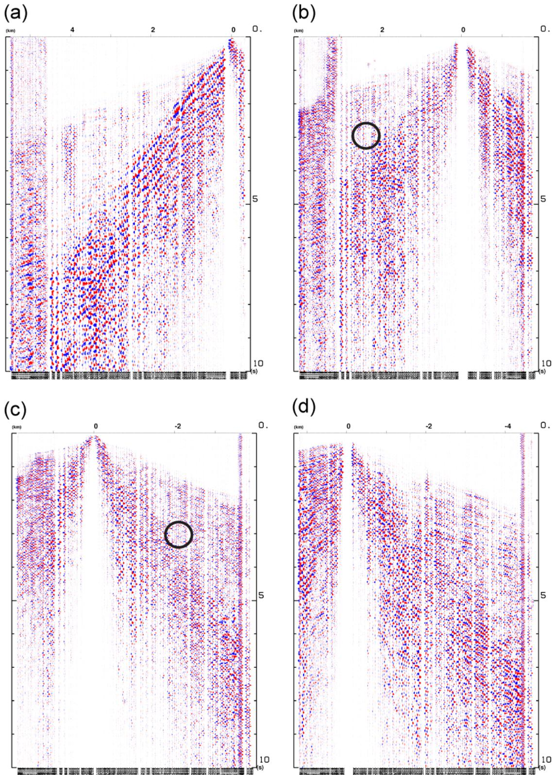
Fig. 2 The 2009 shot records along the line NS. (a) 09S02, (b)09S04, (c)09S12, and (d)09S08. The left end of each plot is for the north end. The location of a shot point is shown 0 km. Each waveform has been normalized at each maximum value. Black circle shows the part which a change can be seen as compared with the last observation in 2008 (Fig. 3).
