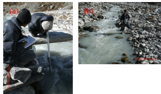
Photo 2 (a) Water depth measurement, (b) Surface water velocity measurement with 14 inch tire tube
