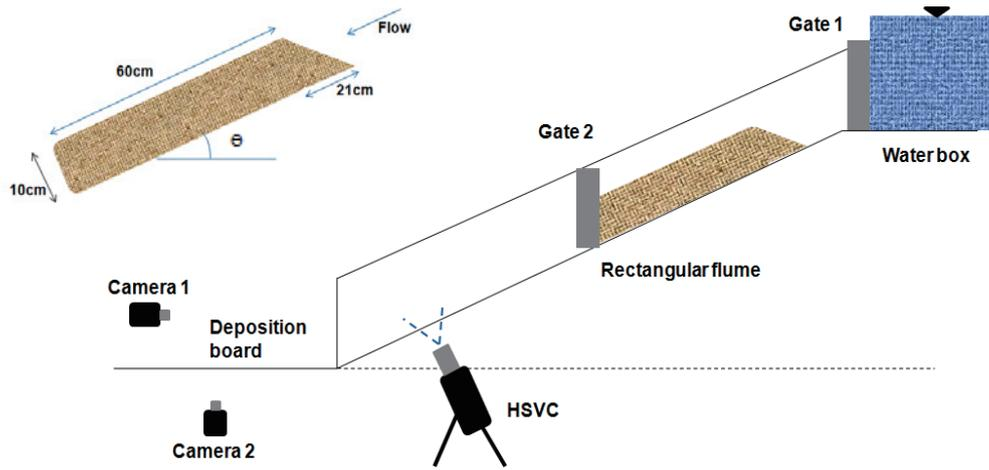
Fig. 2 The diagram of the experimental set-up
