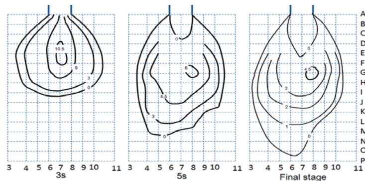
Fig.5 Three stages of debris formation for
