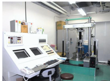
Fig. 9 The stress and pore pressure control ring shear apparatus DPRI-7.
