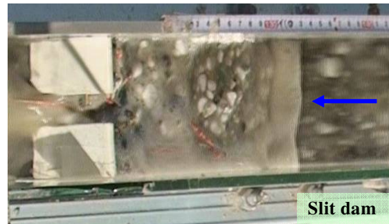
Fig. 16 Flow motion of driftwood at upstream of check dams
