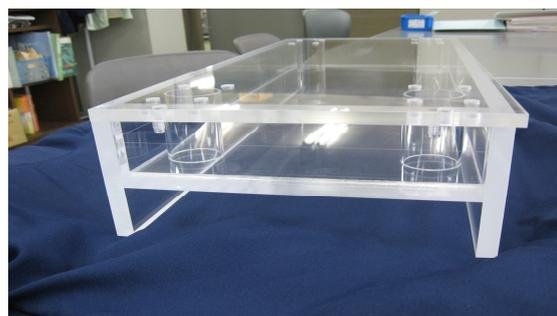
Fig. 2 Double barrier floating breakwater
