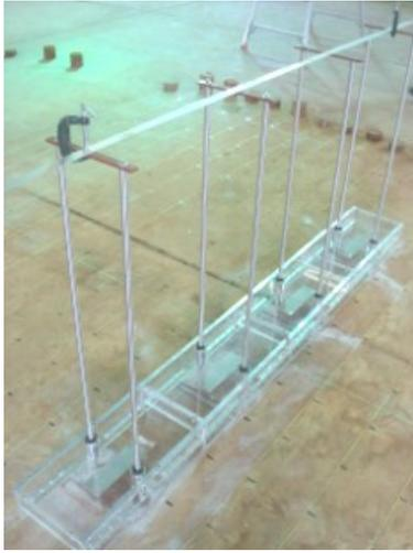
Fig. 7 Double barrier floating breakwater
