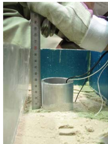
Fig. 5 Uplifted model manhole for CS4
