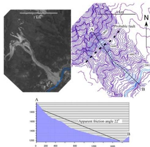
Fig. 5 Long lobate landslide (Xiejiadian landslide, PRISM image, contour map, and a cross section made from the PRISM data).
