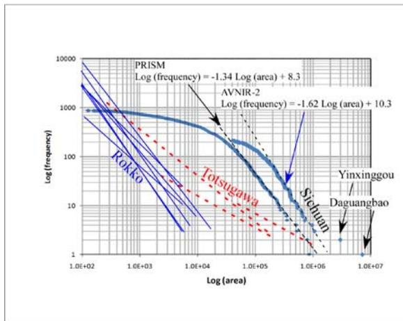
Fig. 13 Cumulative landslide frequency and the landslide size. Data of Rokko and Totsugawa are from Hirano and Ohmori (1989). Rokko and Totsugawa is a granite and Cretaceous sedimentary rock area, respectively.
