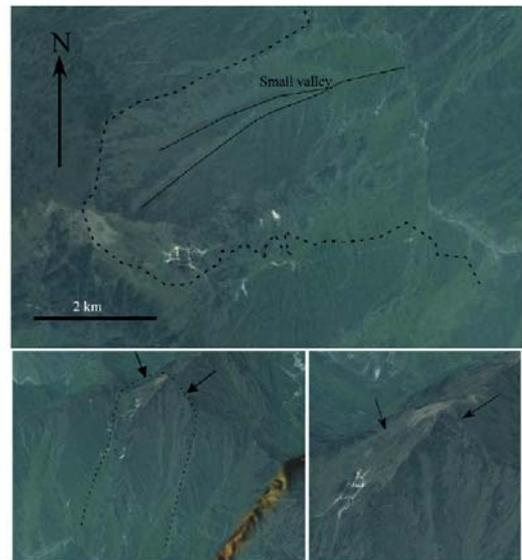
Fig. 9 Outline of Daguangbao landslide and linear depressions (arrows) at the top of the landslide area before the slide (Google Earth). Lower two photographs are oblique views of the linear depressions looked from NE.
