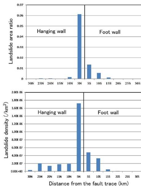
Fig. 12 Landslide distribution histogram according to the distance from the fault surface rupture between Beichuan and Pingdong.
