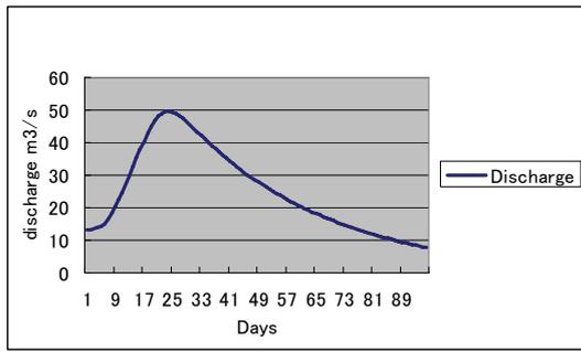
Fig. 17 Hydrograph of hourly discharge simulation
