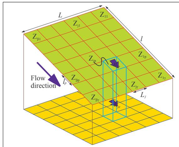
Fig. 5 Schematic diagram showing the homogenization method Fig. 5 Schematic diagram showing distribution of the slope direction cells and the transverse cells (as two dimensional domain), where slope direction:  $\gamma$ , vertical direction:  $\beta$ , slope length:  $l$ (m), slope width:  $L$ (m), cell  $Z_{jp}$ , Size :  $L_j$ (m) $\times$  $l_p$  (m), coefficient of roughness:  $n_{jp}$ ( $m^{-1/3}$  .s), and coefficient of permeability:  $k_{jp}$ (m/s) (Hamaguchi *et. al.*, 2007).
