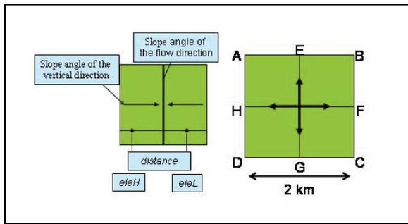
Fig. 8 Schematic diagram of the flow direction determination
