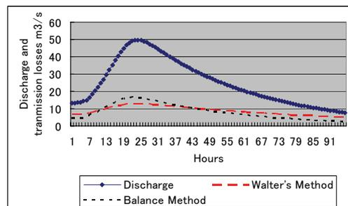
Fig.21 Comparing of discharge and transmission losses (Walter's Equation and Balance method)
