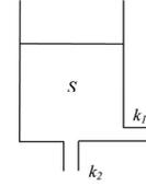
Where  $S$ : is storage amount [ $m$ ],  $I$ : is inflow [ $ms^{-1}$ ],  $O$ : is outflow [ $ms^{-1}$ ],  $k_1$ ,  $k_2$ : are coefficient of permeability
