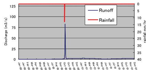
Fig.16 Daily discharge simulation hydrograph and rainfall hyetograph.
