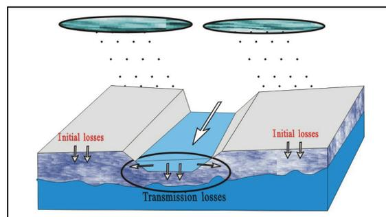
Fig.2 Conceptual model showing transmission and initial losses in the Wadi System
