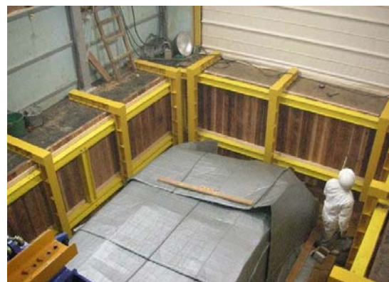
Photo 5 Layout of Earth Retaining Walls
