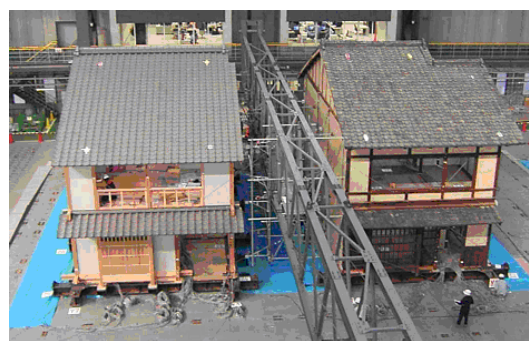
Photo 4 Shaking table test of two Kyo-machiya houses (Left: new house, Right: old house)
