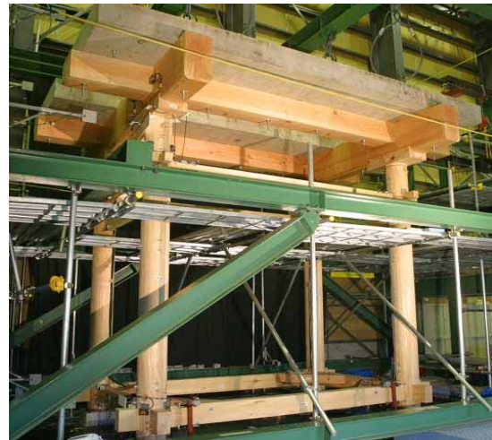
Photo 10 Specimen C without bracket complex
