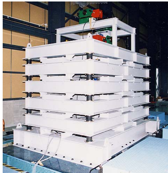
Photo 1 Test frame for shaking table test
