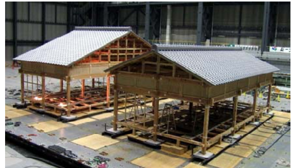
Photo 8 Specimens with tiled roof
