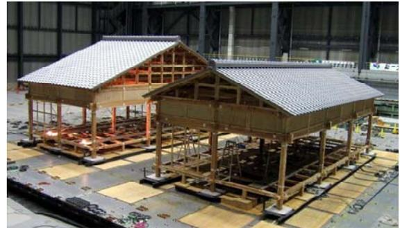
Photo 8 Specimens with tiled roof
