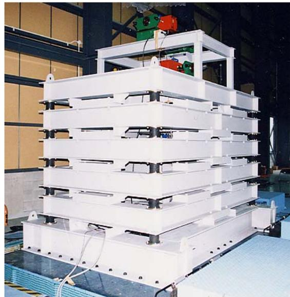
Photo 1 Test frame for shaking table test
